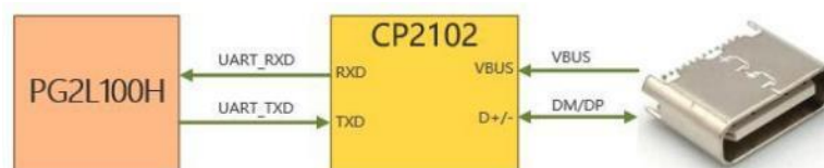
Figure 3-3 USB-UART Block Diagram
